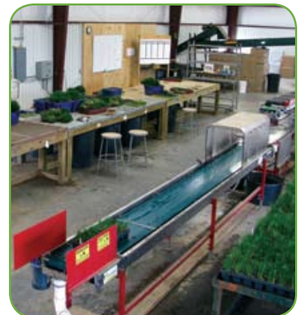
The sticking line for ornamental grass divisions at Hoffman Nursery in Rougemont, N.C., is simple and without a lot of automation. Clumps of grasses are divided on the wooden benches across from the sticking line.
